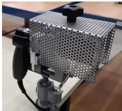
EArgo tool plate protection, protection holder and bench vise
